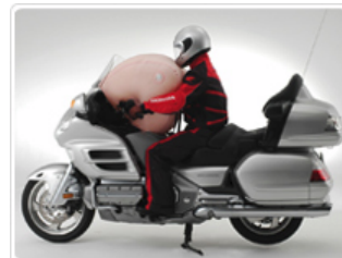
Honda's motorcycle airbag system, the first of its kind
