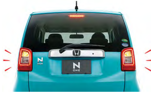
Emergency Stop Signal: The hazard lamps automatically start flashing quickly in the event of abrupt braking.
